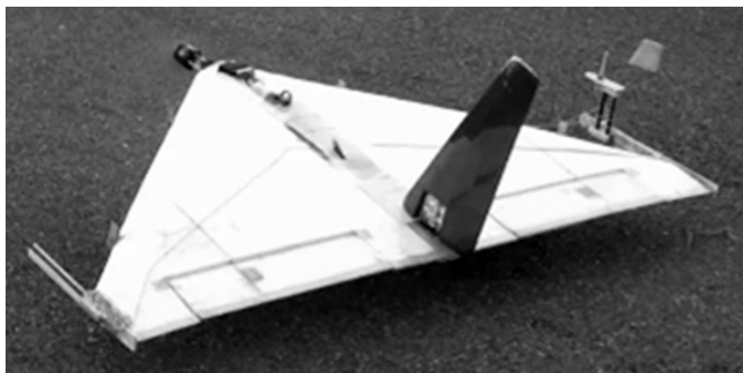
Figure 2. Photograph representing instrumented prototype of CDRW configuration 14 .
