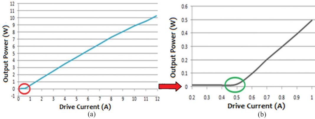
Figure 3. (a) P-I Characteristics and (b) Threshold region.
