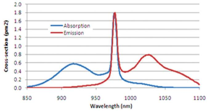
Figure 5. Active fiber with absorption and emission spectrum.
