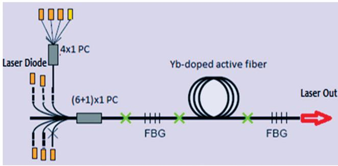
Figure 8. Basic optical scheme of fiber laser.
