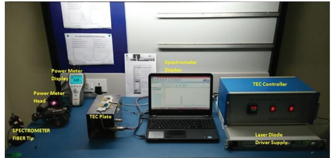
**Figure 2. Experimental set-up.**
