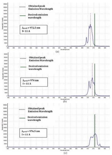
Figure 6. Emission spectrum at (a) 15 °C, (b) 20 °C, and (c) 25 °C.
