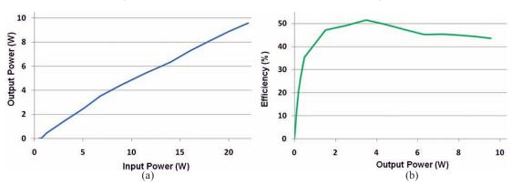
Figure 4. (a) Output power vs input power and (b) Efficiency vs output power.
