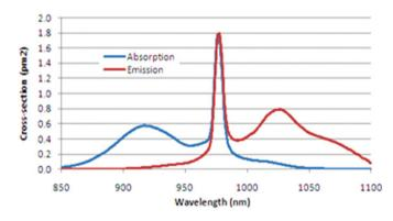
Figure 5. Active fiber with absorption and emission spectrum.
