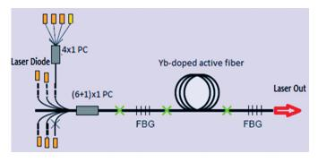
Figure 8. Basic optical scheme of fiber laser.
