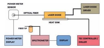
Figure 1. Schematic of an experimental setup used for evaluation of laser diode.
