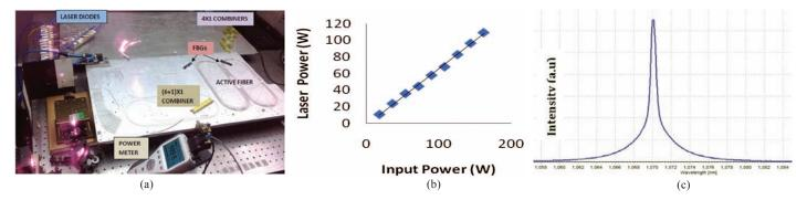
Figure 10. (a) Experimental setup of developed 100 W fiber laser, (b) Laser power vs pump power, and (c) Output spectrum.
