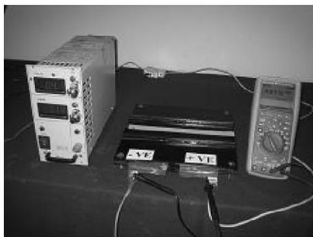
Figure 2. Experimental set-up for charging.
