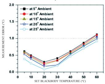
Figure 5. Absolute measurement error for MWIR camera after re-calibration.
