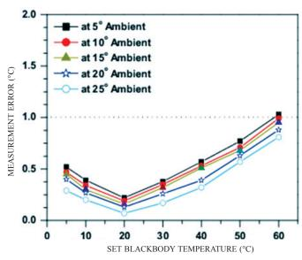
Figure 6. Absolute measurement error for LWIR camera after re-calibration.
