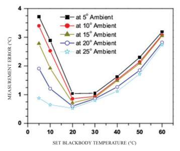
Figure 3. Absolute measurement error for MWIR camera at variable ambient temperature.
