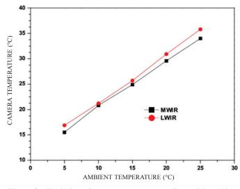
Figure 2. Variation of camera temperature  $(T_{Cam})$  with ambient temperature.
