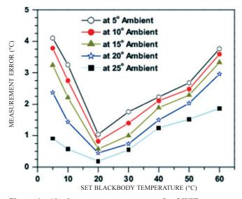
Figure 4. Absolute measurement error for LWIR camera at variable ambient temperature.
