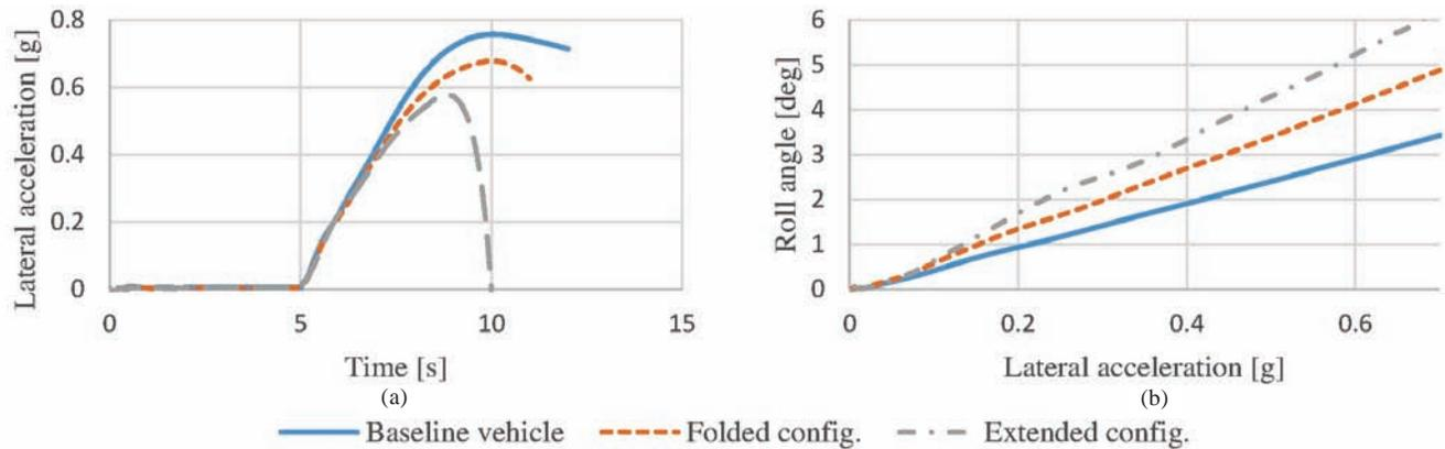
Figure 7. Simulation results of the ramp steer event.
