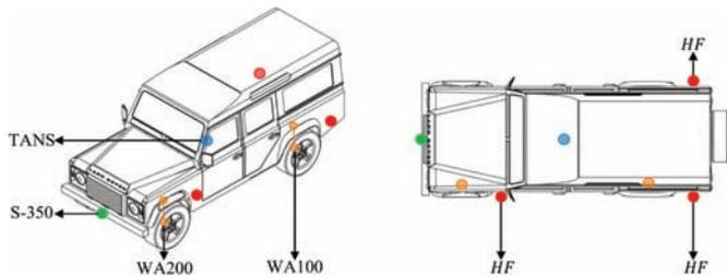
Figure 3. Vehicle measurement positions.
