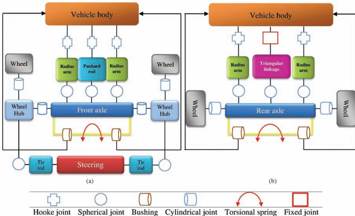
**Figure 2. Kinematic schemes of the suspension systems: (a) front suspension and (b) rear suspension.**
