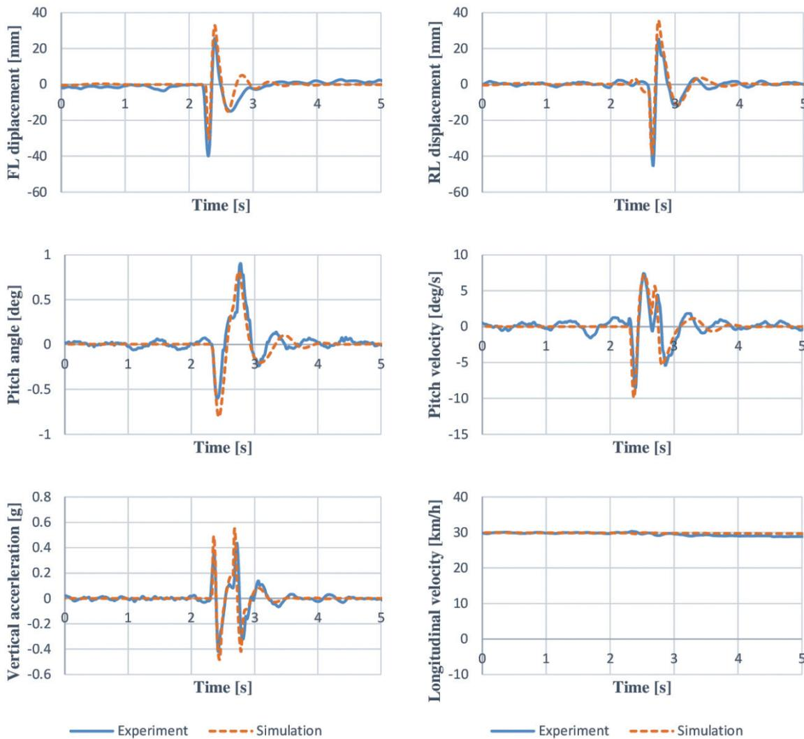
Figure 4. Simulation and experimental results for a bump test at 30 km/h.
