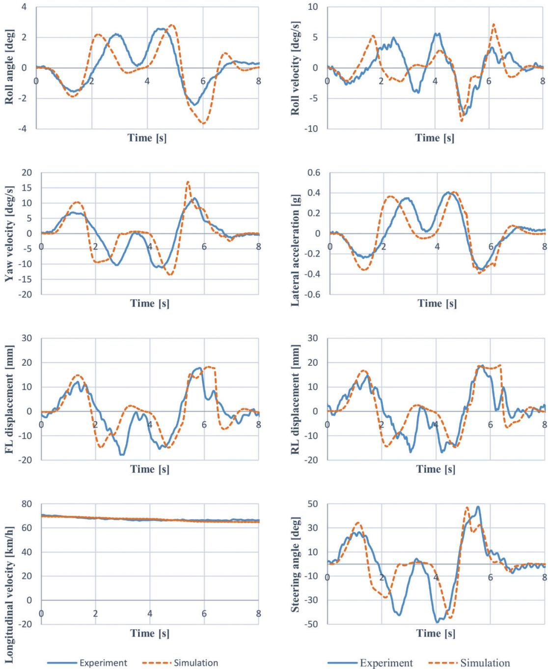
Figure 5. Simulation and experiment results for a double lane change manoeuvre at 70 km/h.
