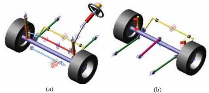
**Figure 1. MSC.ADAMS/Car full vehicle model. (a) front suspension and steering and (b) rear suspension.**
