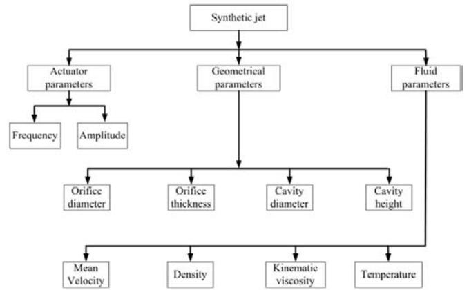
**Figure 2.** Parameters governing the synthetic jet.
