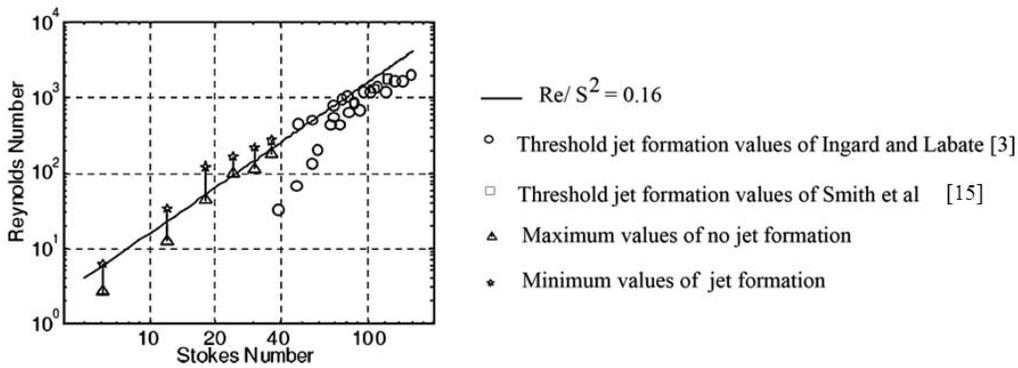
Figure 4. SJ formation criterion for axisymmetric case<sup>14</sup>.
