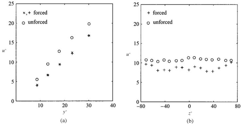
Figure 6. Mean velocity<sup>24</sup> (a) wall normal direction at  $x^+=10$  (b) spanwise direction at  $y^+=15$ .
