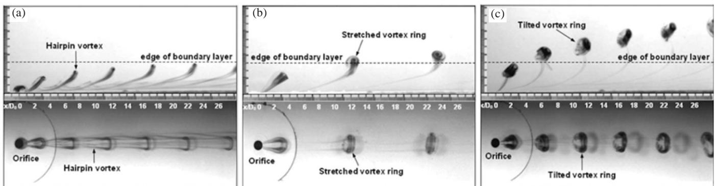
Figure 7. (a) Hairpin vortices, (b) Stretched vortex rings, and (c) Tilted vortex rings<sup>29</sup>.
