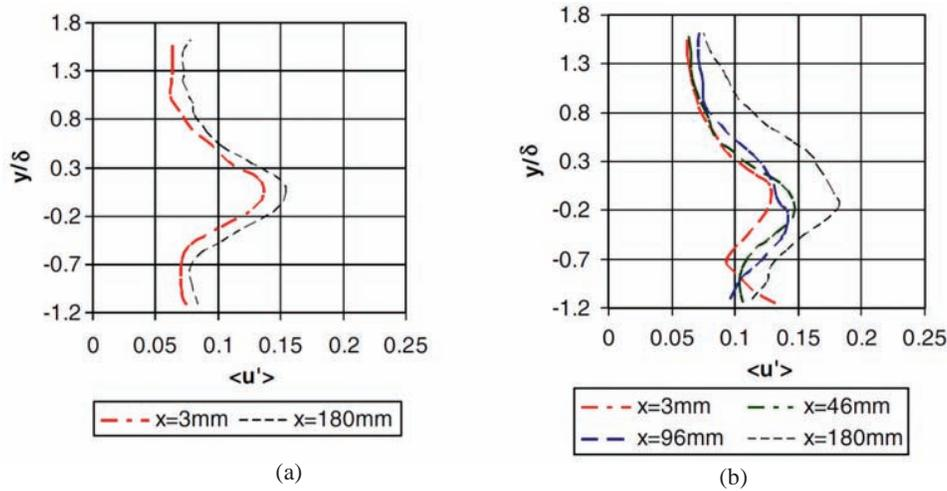
Figure 10. Streamwise velocity fluctuations (a) uncontrolled (b) controlled flow<sup>36</sup>.
