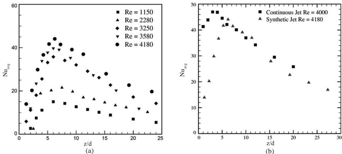
Figure 12. (a) Nu variation with axial distance (b) Nu for synthetic and continuous jet<sup>45</sup>.
