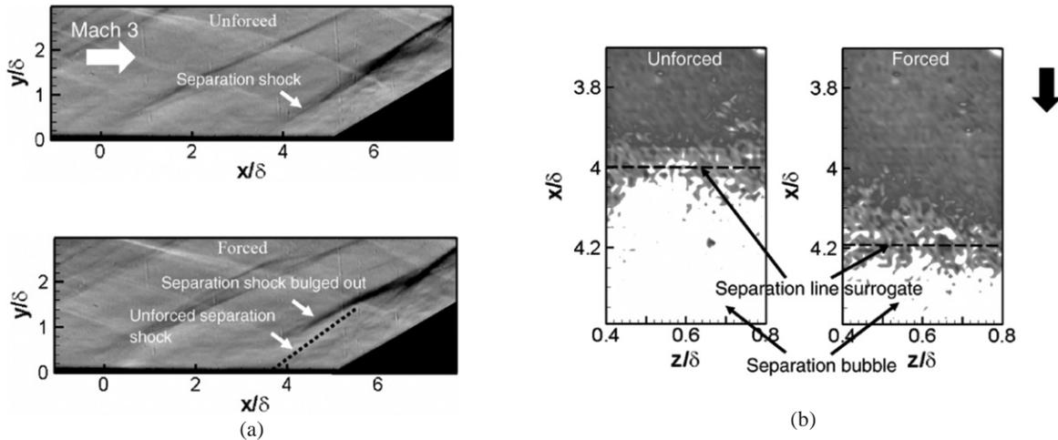
Figure 8. (a) Schlieren (b) phase-locked planar laser scattering (PLS) images showing the separation-scale reduction<sup>32</sup>.
