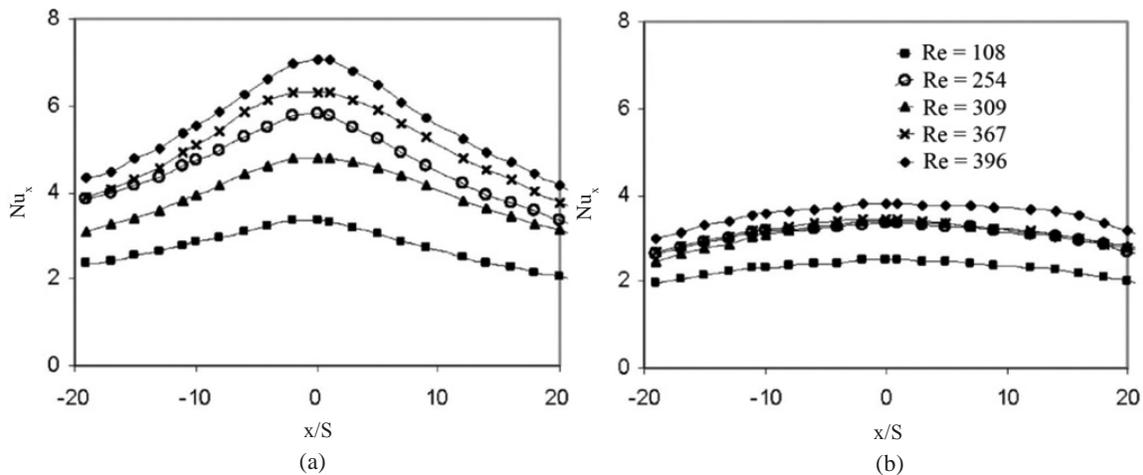
Figure 11. Spanwise distributions of Nu at the normalised spacing of (a) 14.5 and (b) 22.7<sup>41</sup>.
