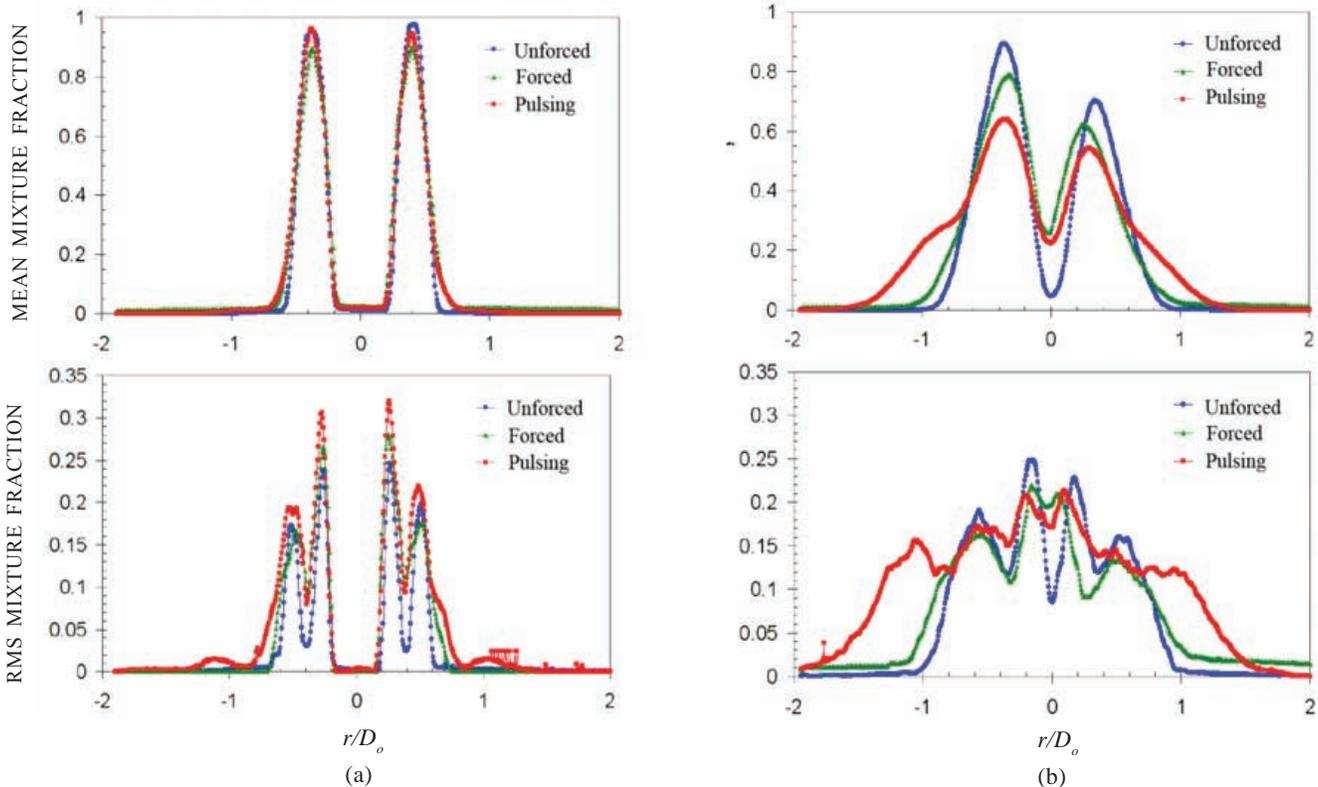
Figure 9. Comparison of mean and rms mixture fraction profiles (a)  $x/D_o=0.25$  (b)  $x/D_o=2$ <sup>34</sup>.
