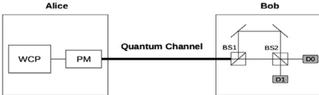
**Figure 1. Block diagram of DPS (differential phase shift) QKD protocol.**
