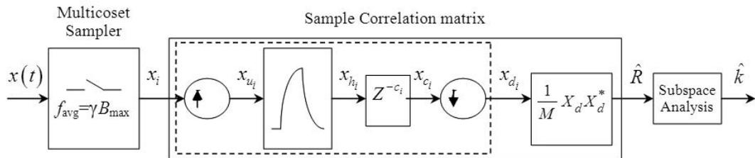
Figure 2. The block diagram for broadband spectrum sensing system.
