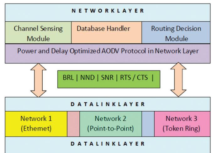
Figure 2. Functional Block diagram of cross layer interaction.
