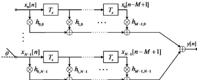
Figure 1. Wideband beamforming by space-time processor.
