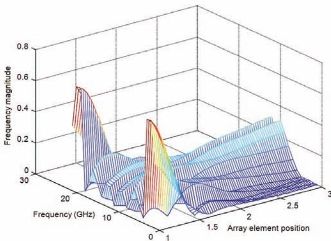
Figure 3. Frequency magnitude of FIR filters.
