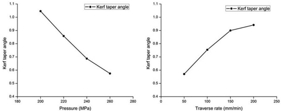
Figure 3. Effect of pressure and traverse rate on kerf taper.
