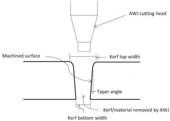
Figure 1. Schematic illustration of kerf geometry.
