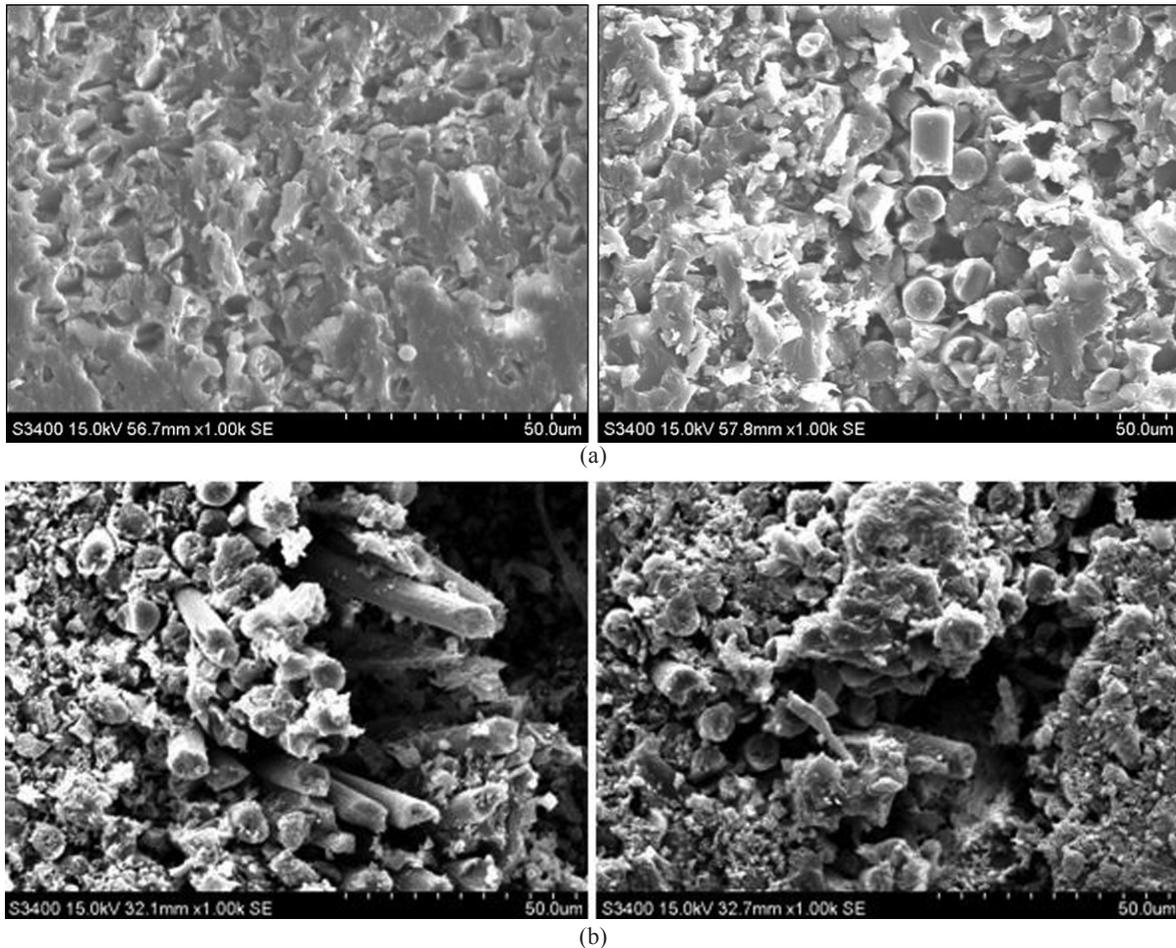
Figure 4. Machined surfaces of (a) sample 1 and sample 2, (b) sample 3 and sample 4 (Horizontal surface at 1000x).
