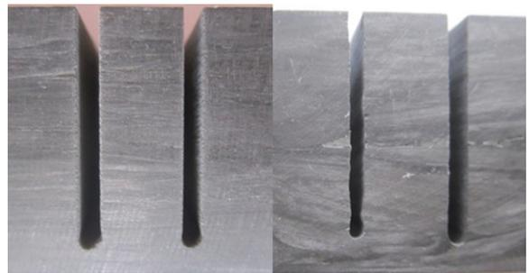
Figure 5. Top and bottom kerf edges.
