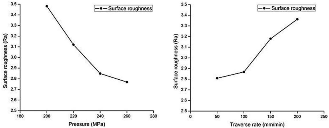
Figure 2. Effect of pressure and traverse rate on surface roughness.
