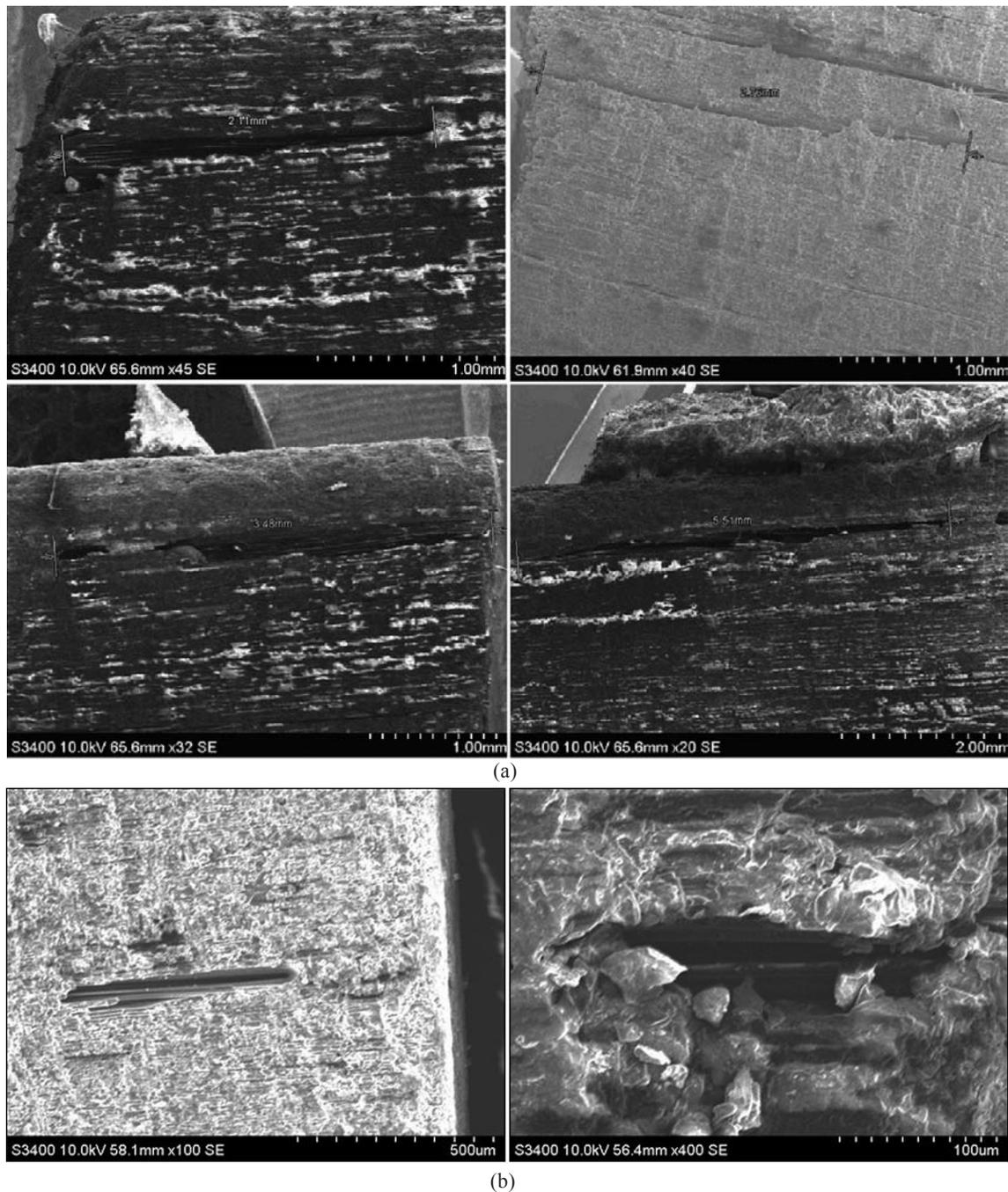
**Figure 6. (a) Delamination in machined samples and (b) Fibre pull out and abrasive embedment.**
