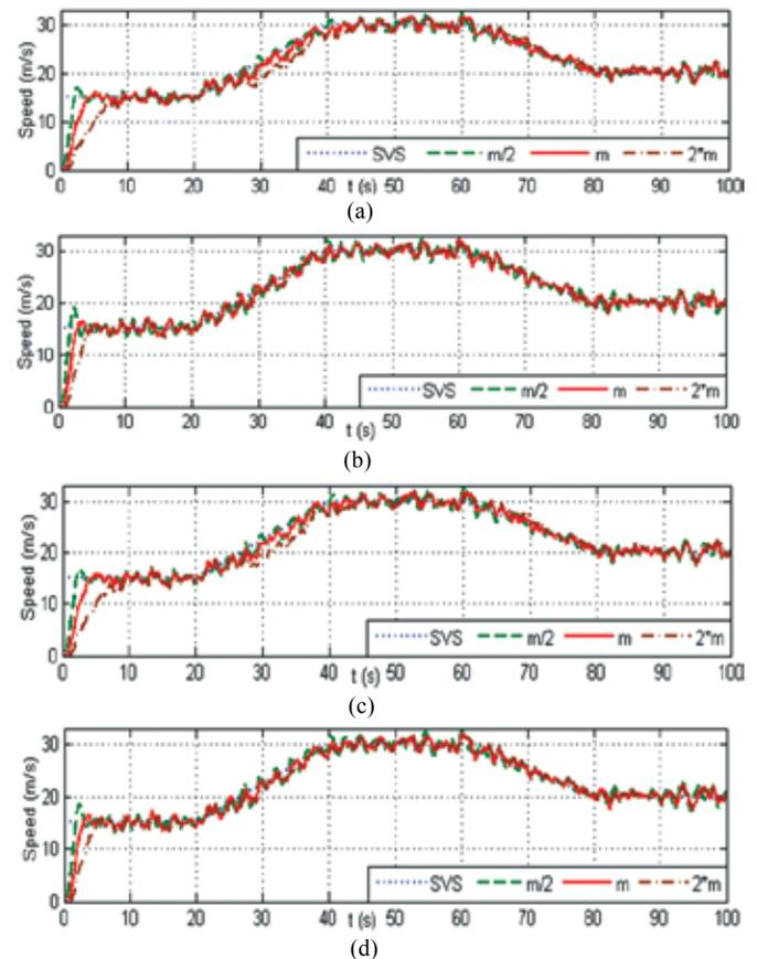
Figure 12. Response of speed under non-deterministic road grade, noise and uncertainty in mass ; (a) ANN based I-IMC without adaptive control, (b) ANN based I-IMC with adaptive control, (c) ANFIS based I-IMC without adaptive control, (d) ANFIS based I-IMC with adaptive control.
