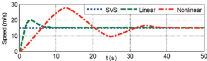
Figure 3. Speed response of HDV system with S-IMC.
