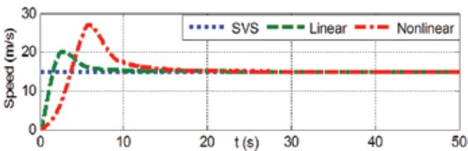
Figure 4. Speed response of HDV system with I-IMC.
