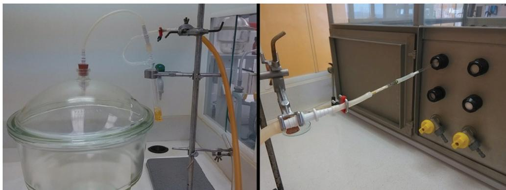
Figure 1. Sampling followed by spectrophotometric determination of chlorine concentration in the desiccator (left) and collection of sample from the 617 dm<sup>3</sup>-in-vol chamber
