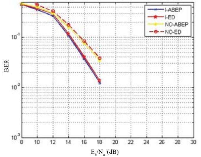
Figure 6. Comparison of detectors in the presence of NBI and after mitigating NBI w.r.t.  $E_b/N_0$ .
