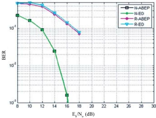
Figure 4. Comparison of Nyquist Rate and reconstruction based energy detectors w.r.t.  $E_b/N_0$ .
