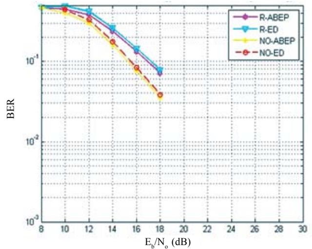
Figure 7. Comparison of detectors in the absence of NBI and after notching out NBI w.r.t.  $E_b/N_0$ .
