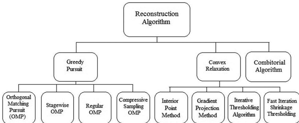
Figure 2. Classifications of reconstruction algorithms in CS theory.
