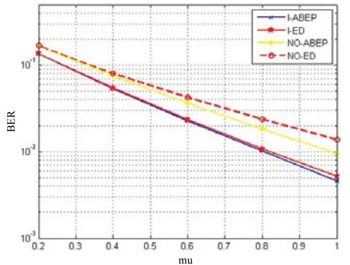
Figure 8. Comparison of Nyquist rate energy detector and compressed sampling based energy detector w.r.t.  $\mu$ .
