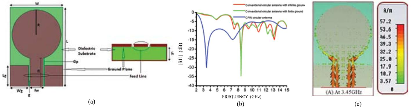
Figure 1. (a) Geometry of CPW fed circular patch antenna with its parameter, (b) Comparison of variation of  $|S_{11}|$  with frequency of circular patch antenna in different cases, and (c) Current distribution at 3.45 GHz.
