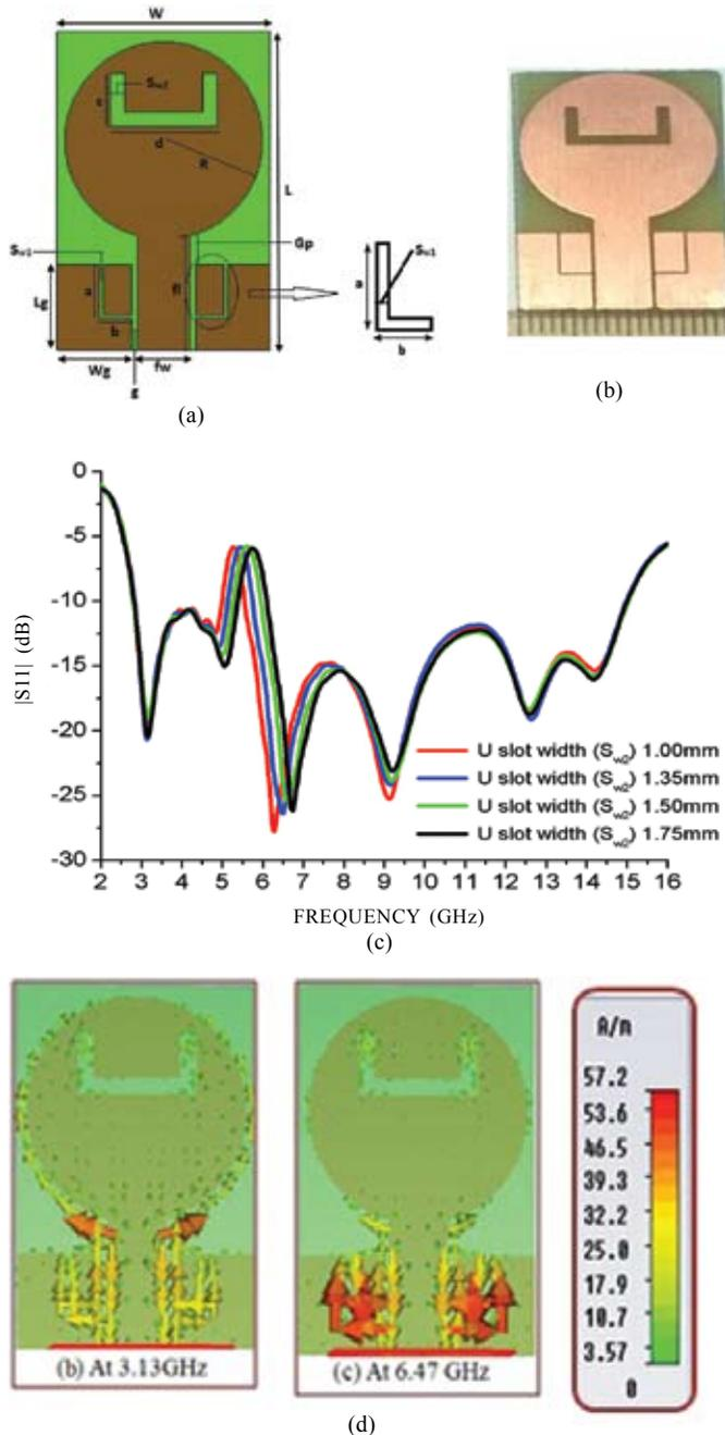
**Figure 5.** (a)-(b) Geometry of CPW fed circular patch antenna with U shaped slot in patch, (c) Comparison of variation of  $|S_{11}|$  with frequency of circular patch antenna for different U slot width, and (d) Current distribution at different resonance frequencies.
