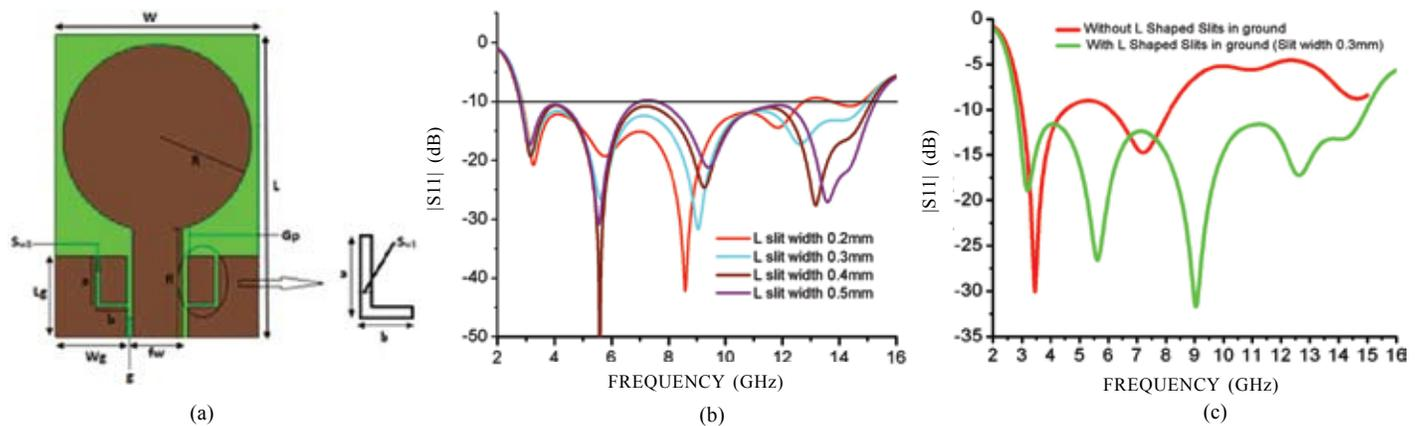
Figure 2. (a) Geometry of CPW fed circular patch antenna with L shaped slits in ground plane, (b) Comparison of variation of  $|S_{11}|$  with frequency of circular patch antenna for different slit thickness, and (c) Comparison of variation of  $|S_{11}|$  with frequency of patch antenna with and without L shaped slits in ground plane.
