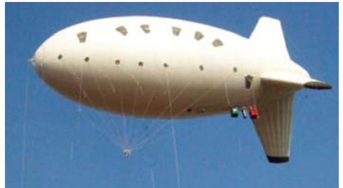
**Figure 12. Envelope in tethered condition.**
