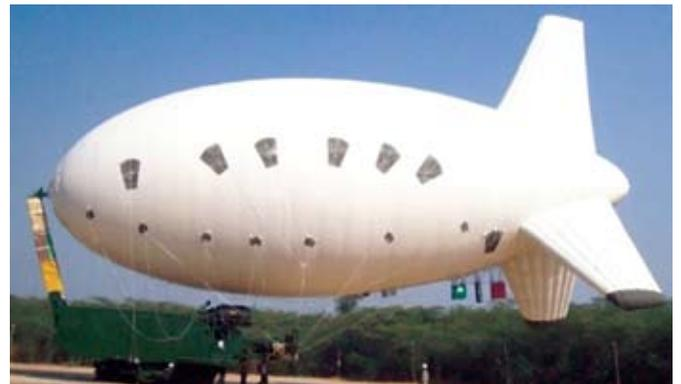
**Figure 13. Envelope in mooring condition.**
