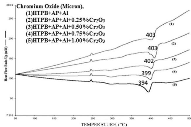
**Figure 9. Effect of micron sized Cr<sub>2</sub>O<sub>3</sub> on thermal decomposition of composite propellant formulation.**
