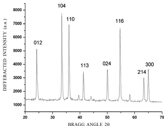
Figure 3. X-ray diffraction pattern of micron  $\text{Cr}_2\text{O}_3$ .
