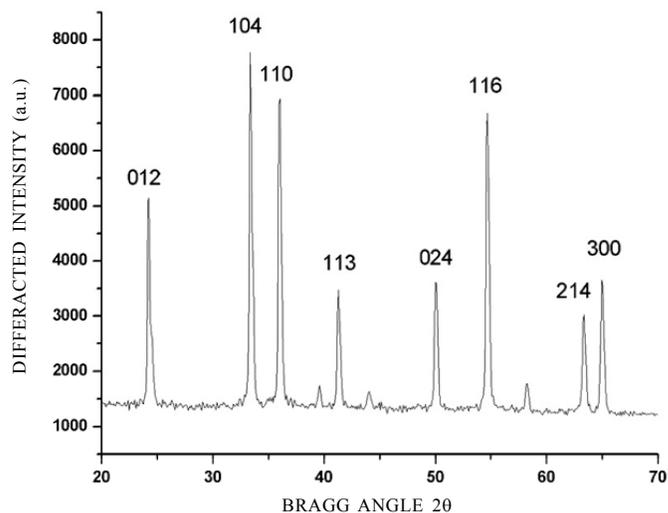
Figure 2. X-ray diffraction pattern of nano- $\text{Cr}_2\text{O}_3$ .
