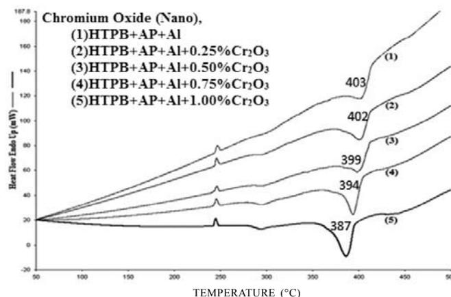
**Figure 8. Effect of nano sized Cr<sub>2</sub>O<sub>3</sub> on thermal decomposition of composite propellant formulation.**
