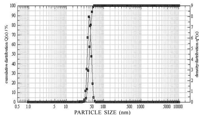
Figure 1. Particle size distribution of nano-  $\text{Cr}_2\text{O}_3$ .
