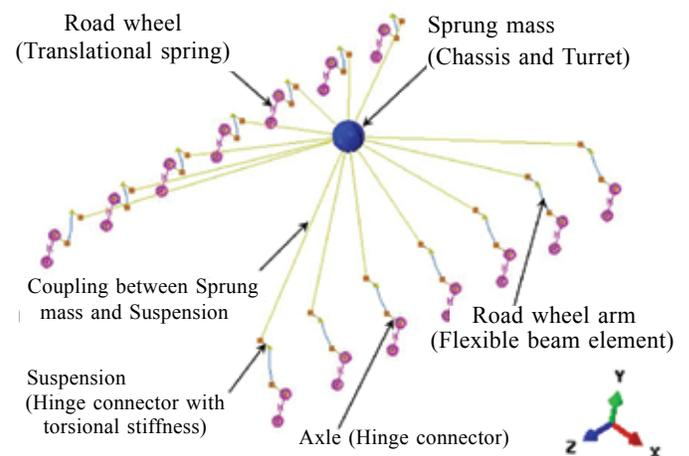
Figure 4. Equivalent model with flexible road wheel arm.
