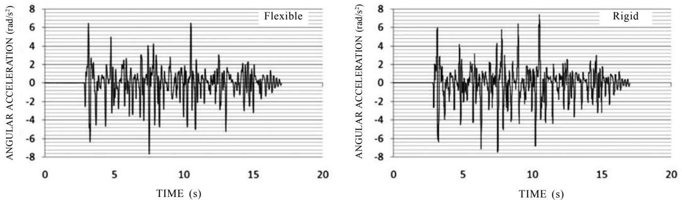
Figure 10. Pitch angular acceleration of sprung mass CG (about X-axis).
