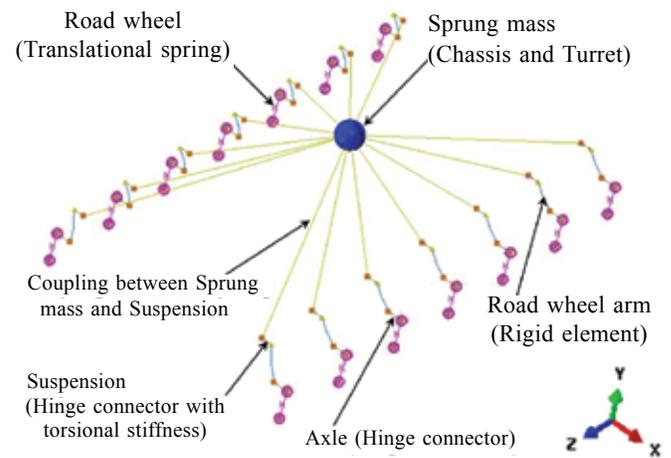
Figure 3. Equivalent model with rigid road wheel arm.
