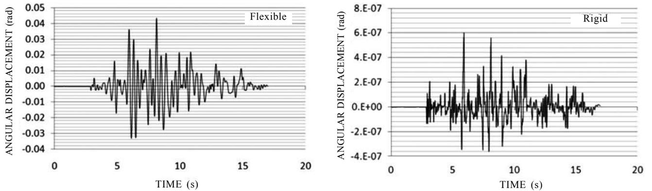
Figure 13. Roll angular displacement of sprung mass CG (about Z-axis).
