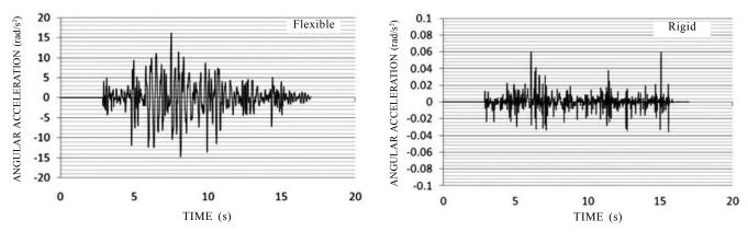
Figure 14. Roll angular acceleration of sprung mass CG (about Z-axis).
