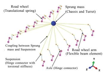
Figure 4. Equivalent model with flexible road wheel arm.
