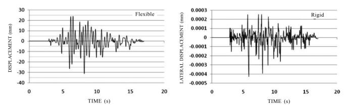
Figure 11. Lateral displacement of sprung mass CG (along X-axis).
