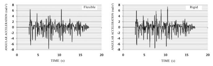
Figure 10. Pitch angular acceleration of sprung mass CG (about X-axis).
