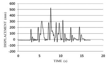
Figure 6. Vertical wheel displacement data.
