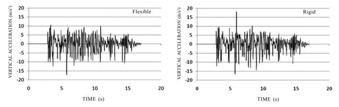
Figure 8. Vertical acceleration of sprung mass CG (along Y-axis).
