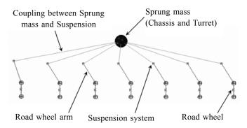
Figure 2. Equivalent tracked vehicle model.
