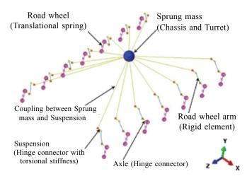
Figure 3. Equivalent model with rigid road wheel arm.
