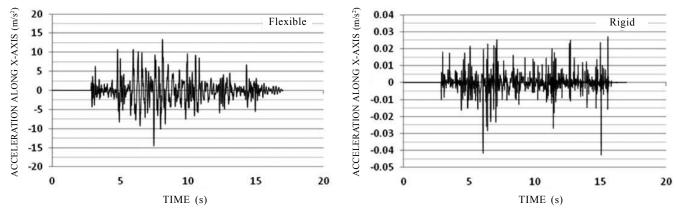
Figure 12. Lateral acceleration of sprung mass CG (along X-axis).
