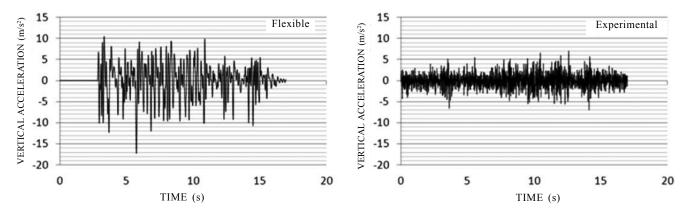
Figure 15. Vertical acceleration of flexible vehicle model and the actual vehicle.
