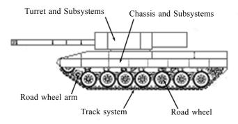
Figure 1. Schematic tracked vehicle configuration.
