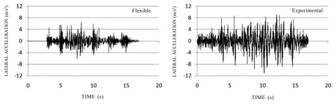
Figure 16. Lateral acceleration of flexible vehicle model and the actual vehicle.
