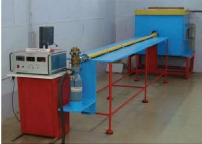
Figure 1. Compressed air gun test setup.
