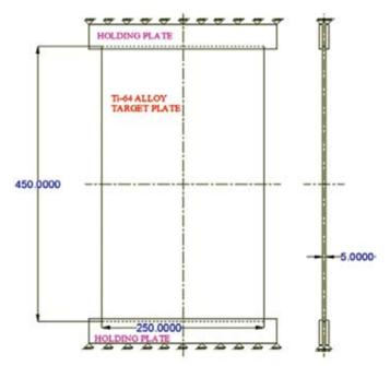
Figure 2. Geometric model of flat plate.
