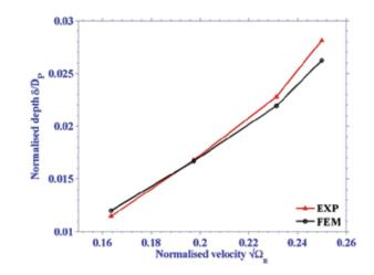
Figure 7. Variation of residual depth with impact velocity.
