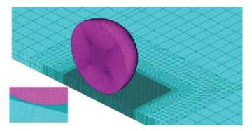
Figure 4. Symmetrical model of titanium specimen with spherical projectile.
