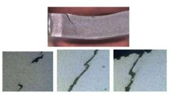
Figure 10. Deformation by shear band formation at velocity 75 m/s.
