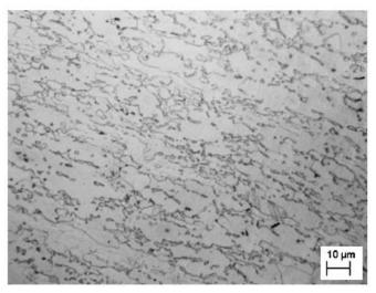
Figure 3. Microstructure of the plate along rolling and impact directions.
