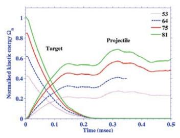
Figure 5. Temporal variation in normalised kinetic energy of projectile and target at different impact velocities.
