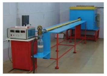
Figure 1. Compressed air gun test setup.
