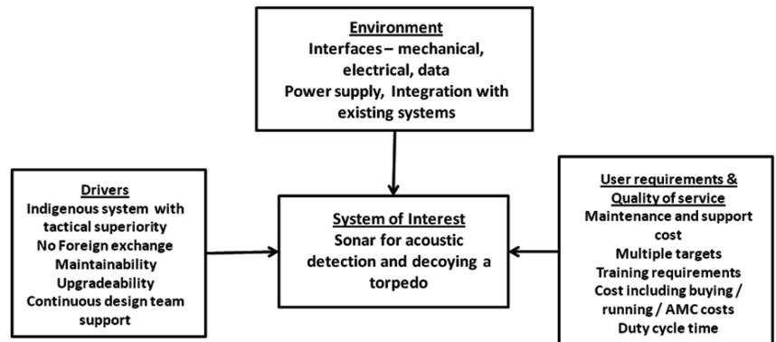
Figure 3. Context diagram for a torpedo defence system.
