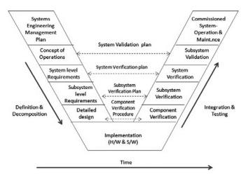
Figure 1. The V diagram in systems engineering.
