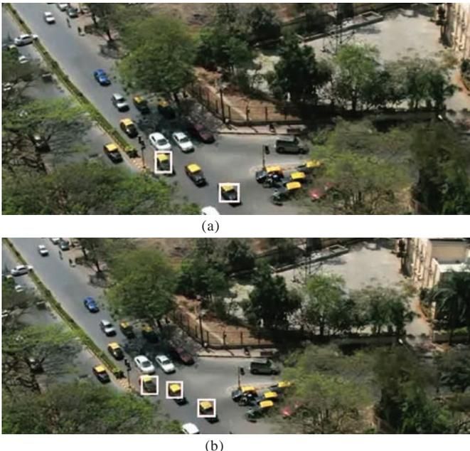
Figure 10. (a) Frame 24 – Tracking object of interest (middle taxi) failed and (b) Frame 24 - The object of interest is tracked accurately with distance measure cue.
