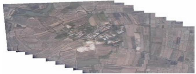
Figure 4. A panoramic image registered by UAV video image sequence.
