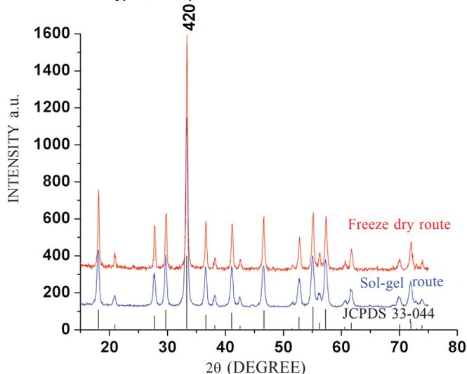
Figure 1. XRD of Nd:YAG nanopowder on calcination at 1000 °C for 2 h.
