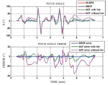
Figure 9. Comparison of MEKF results with NCF for pitch angle.
