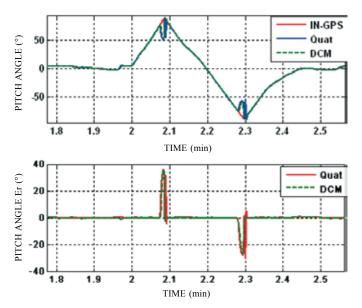
Figure 7. Comparison of MEKF results for pitch angle- case2 (Zoomed for one inverted loop).
