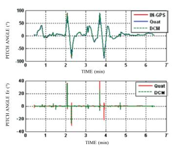
Figure 8. Comparison of MEKF results for pitch angle- case2 (Entire sortie).
