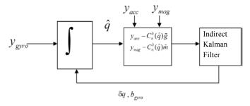
Figure 1. Filter architecture for MEKF.
