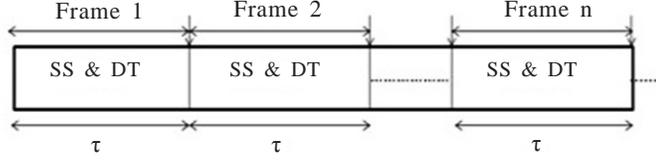
Figure 2. Frame structure for the proposed cognitive radio system<sup>10-12</sup>, SS and DT are spectrum sensing and data transmission time, respectively.
