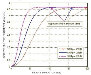
Figure 6. Achievable throughput under various values of SNR<sub>n</sub>.
