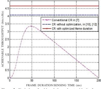
Figure 5. Variation of achieved throughput with the frame duration. Assumed SNR<sub>p</sub> = -20 dB.
