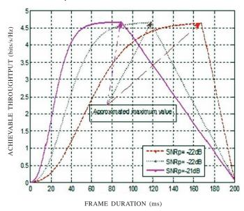
Figure 7. Achievable throughput under various values of SNR<sub>p</sub>. It is assumed that, after time  $\tau^*$ , the PU gets activated with the probability  $P(H_1)=$  0.3 to 0.99.
