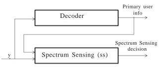
Figure 3. The decoder structure of the proposed CR system<sup>10-12</sup>.
