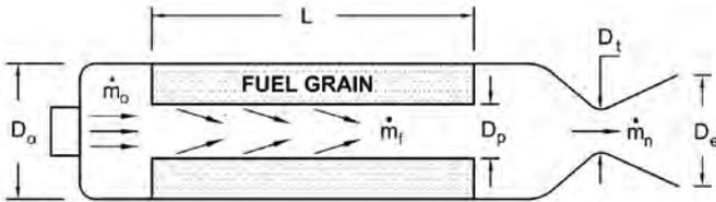
Figure 1. Motor geometry for ballistic model.
