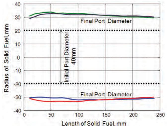
Figure 12. Port diameter variation for test-1A.
