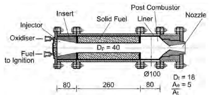
Figure 10. Motor configuration for ignition test 02.
