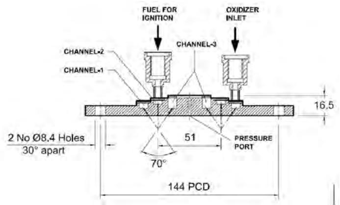
Figure 6. Doublet injector, 4 No. 90° apart.
