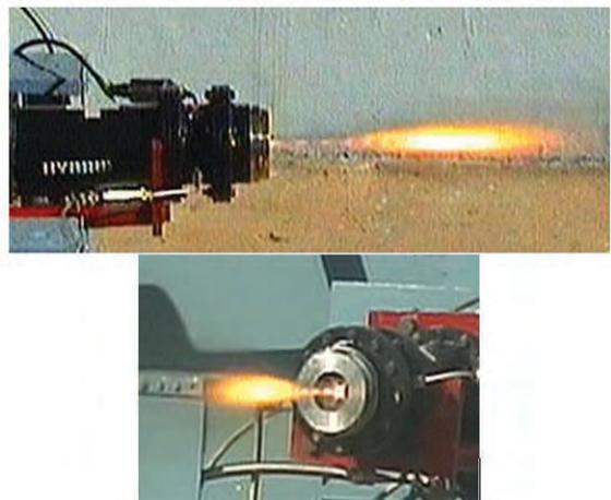
Figure 17. Static test of lab-scale hybrid motor.
