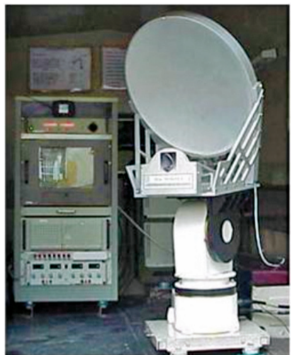
Figure 2. Radiometer sensor test setup.
