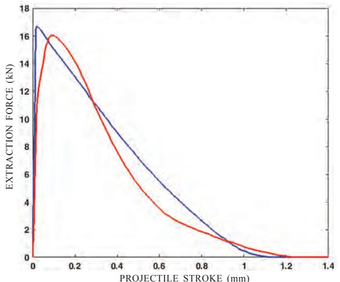
Figure 10. Extraction force from 125 mm barrel.
