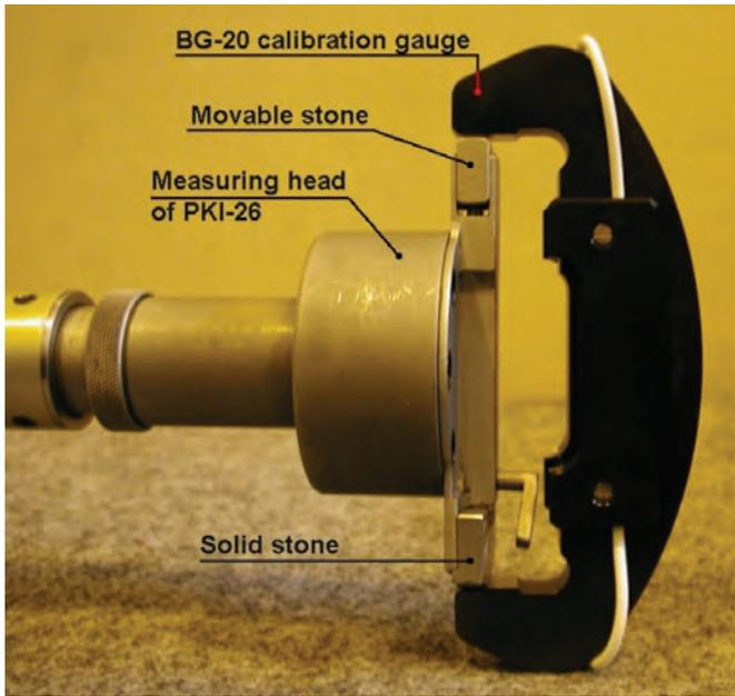
Figure 3. BG20 Calibration gauge as a standard of true value.
