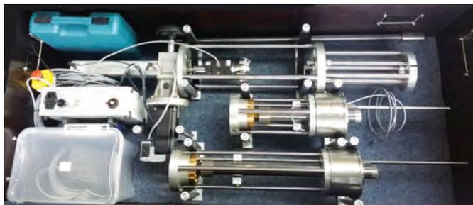
Figure 9. FV-2 semi-automatic measuring device for determination of extraction forces.
