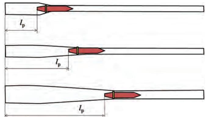
Figure 7. Projectile rammed position in new barrel (above), worn barrel (middle), worn and heated barrel (below).
