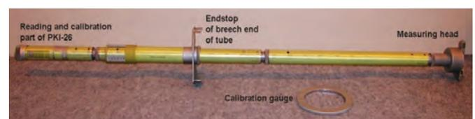
Figure 1. PKI-26 device ready for measurement.
