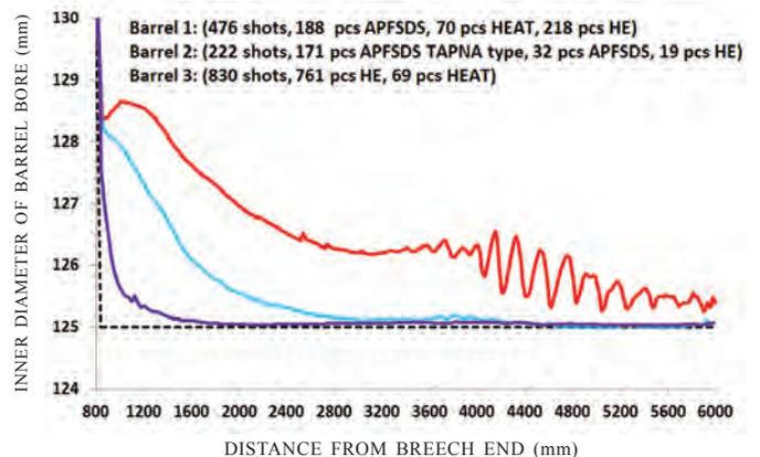
Figure 4. Diameter of guiding parts of worn barrel bores 2A46.
