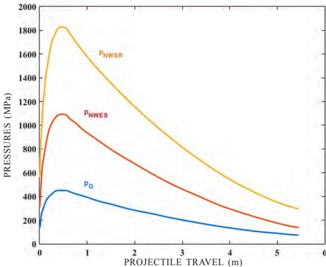
Figure 5. Gas pressure  $p_G$  and contact pressures  $p_{NWES}$ ,  $p_{NWSR}$  depending on projectile path inside of barrel.
