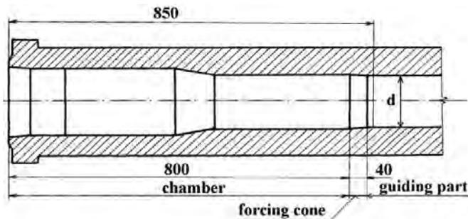
**Figure 8. Parts of smooth barrel bore.**
