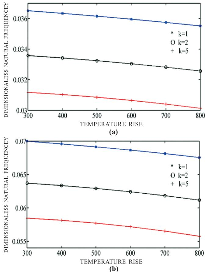
**Figure 2. Dimensionless natural frequency vs temperature rise with nonlinear temperature field for various index values ( $k=1, 2$ , and  $5, k_w=50, k_s=50$ ): (a) First mode and (b) Second mode.**
