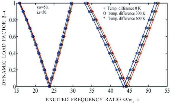
**Figure 6. Dynamic instability regions of FGM plate resting on Pasternak foundation ( $k_w=50, k_s=50$ ), ( $k=1$ ).**
