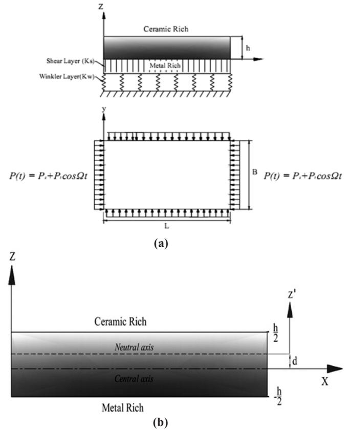
Figure 1. (a) FGM plate resting on elastic foundation and (b) Geometry of the FGM plate.
