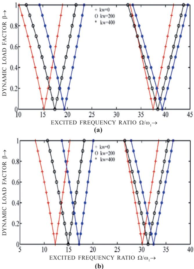
**Figure 7. Effect of Winkler foundation constant on first- and second-mode instability of FGM plate for index values (a)  $k=1$  and (b)  $k=5$ .**
