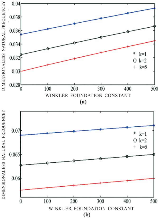
**Figure 3. Effect of Winkler constant on first two frequency parameters ( $k_s=50, \Delta T =200$  K): (a) First mode and (b) Second mode.**
