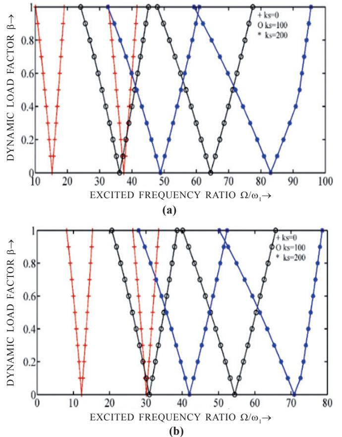
**Figure 8. Effect of Shear layer constant on first- and second-mode instability of FGM plate with index values (a)  $k=1$  and (b)  $k=5$ .**
