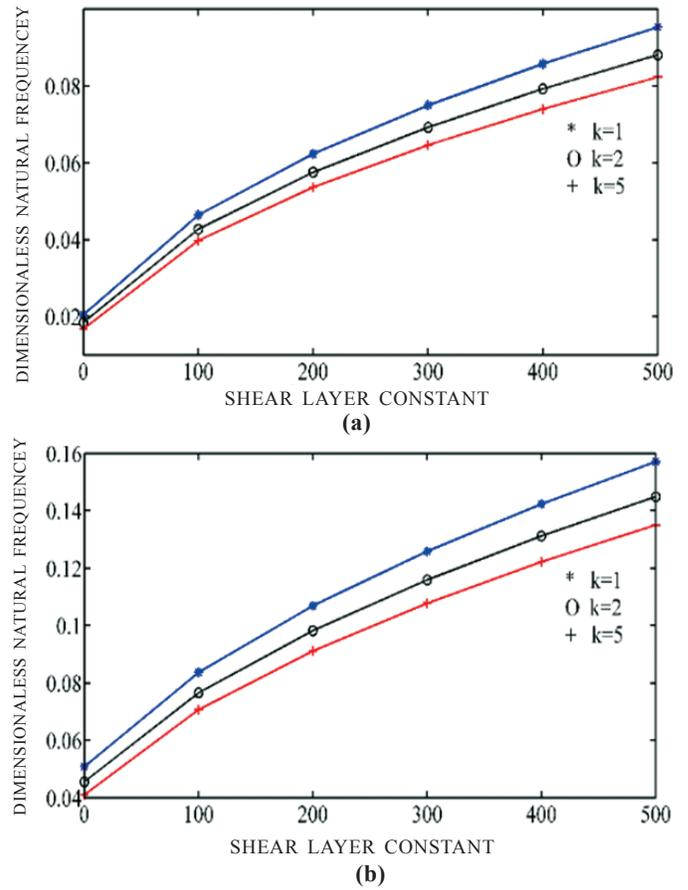
**Figure 4. Effect of shear layer constant on first two frequency parameters ( $k_w=50, \Delta T =200$  K): (a) First mode and (b) Second mode.**
