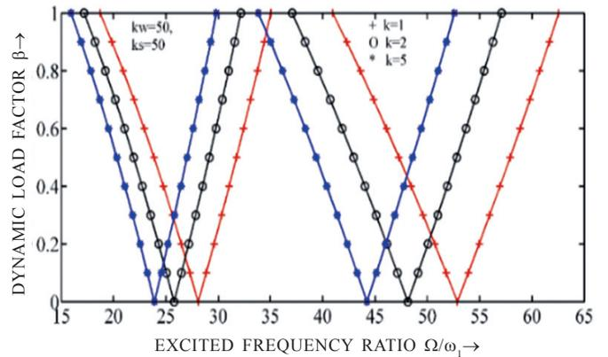
**Figure 5. Regions of instability for first two-mode of FGM plates on Pasternak foundation ( $k_w=50, k_s=50$ ).**
