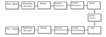
Figure 1. Block diagram of IDMA-OFDM system<sup>2,4</sup>.
