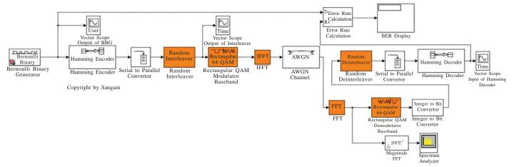
Figure 2. Simulink model of proposed IDMA-OFDM system.
