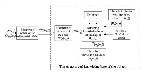
Figure 3. Diagram of an expert system for technical object maintenance.
