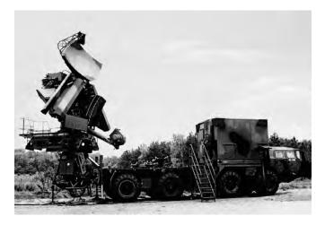
Figure 4. Rocket homing station (NEWA SC) of (SA-3) system. (WZE S.A. photo)
