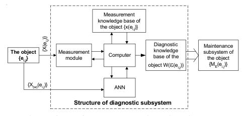
Figure 7. Scheme of measurement module in the diagnostic system.
