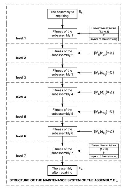
Figure 13. The scheme of structure of the maintenance system of an assembly  $E_{s}$ .
