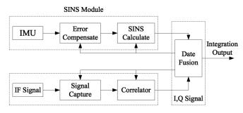
Figure 2. Ultra-tight integration of GPS and IMU.
