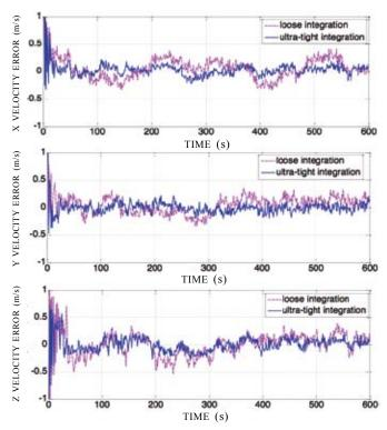
Figure 8. Velocity estimation error statistics.
