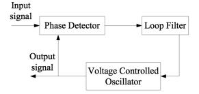
Figure 3. PLL signal process procedure.
