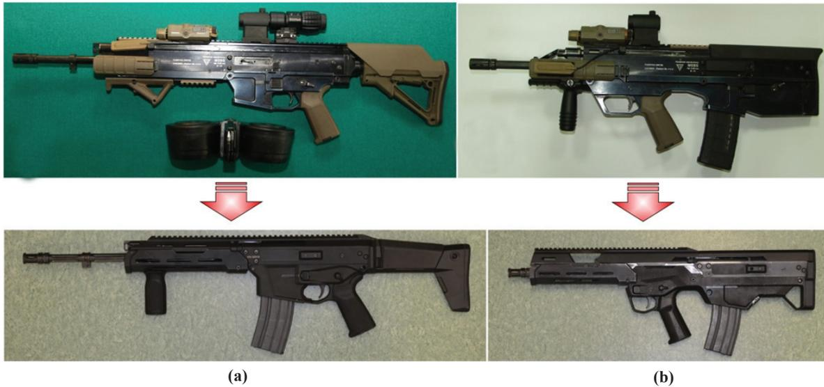
Figure 1. MSBS assault rifles before and after geometrical modifications: (a) classic version and (b) bull-pup version.
