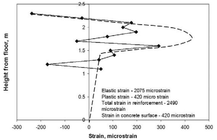
Figure 13. Average strain profile in the left wall.
