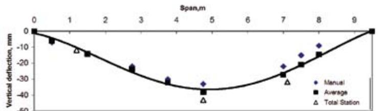
Figure 15. Deflection profile of roof along short span.
