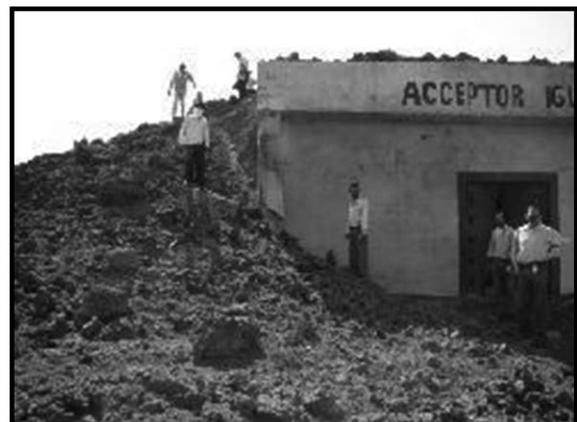
Figure 11. Intact acceptor after trial.
