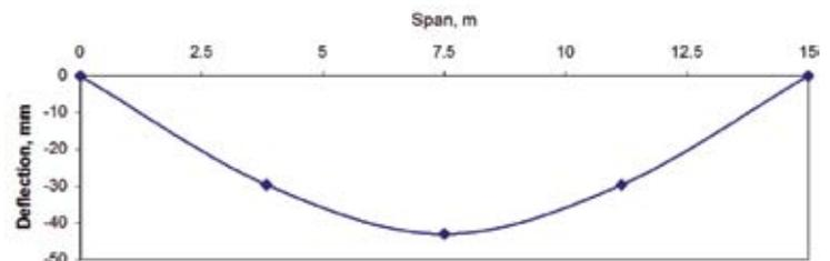
Figure 16. Deflection profile of roof along long span.
