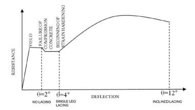
Figure 3. Resistance-deflection curve for flexural reinforced concrete elements.
