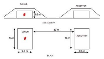
Figure 4. General arrangement of storage structures.
