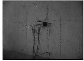
Figure 9. Actual arrangement of targets in left wall.
