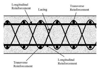
Figure 2. Typical laced reinforced concrete (LRC) structural element.
