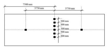
Figure 6. Location of targets (Reflectors) on left wall.
