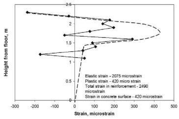
Figure 13. Average strain profile in the left wall.
