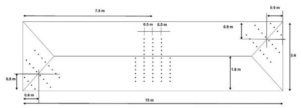
Figure 5. Arrangement of pellets on the inner surface of left wall of acceptor.
