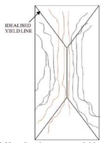
Figure 12. Mapped crack pattern on roof slab of acceptor.
