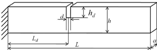
Figure 1. Scheme of the cantilever with the location of the damage.
