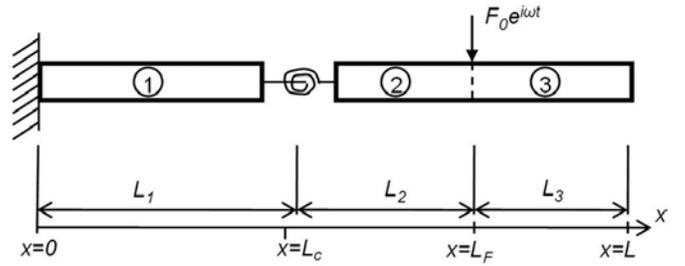
Figure 2. Model of a cantilever beam with an elastic element.
