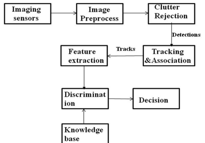
Figure 1. Algorithmic data flow in an ATR system.
