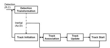
Figure 6. Various stages of Tracking and Association module.
