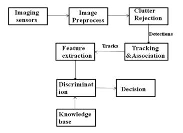
Figure 1. Algorithmic data flow in an ATR system.
