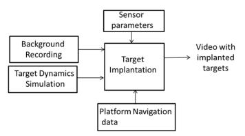
Figure 7. Synthetic data set generation module.
