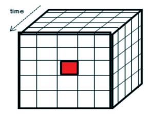
Figure 3. Temporal filtering neighbourhood surrounded by pixel under test.
