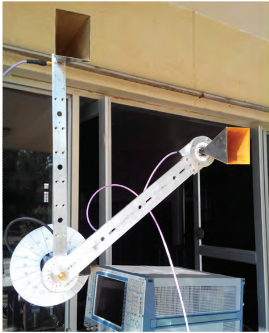
Figure 2. Experimental setup for measurement of scattered radiation.
