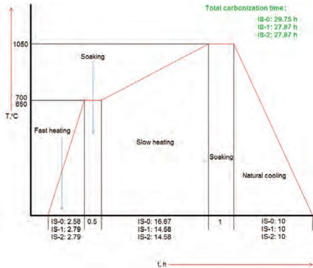
Figure 4. Carbonisation plan for all the samples.
