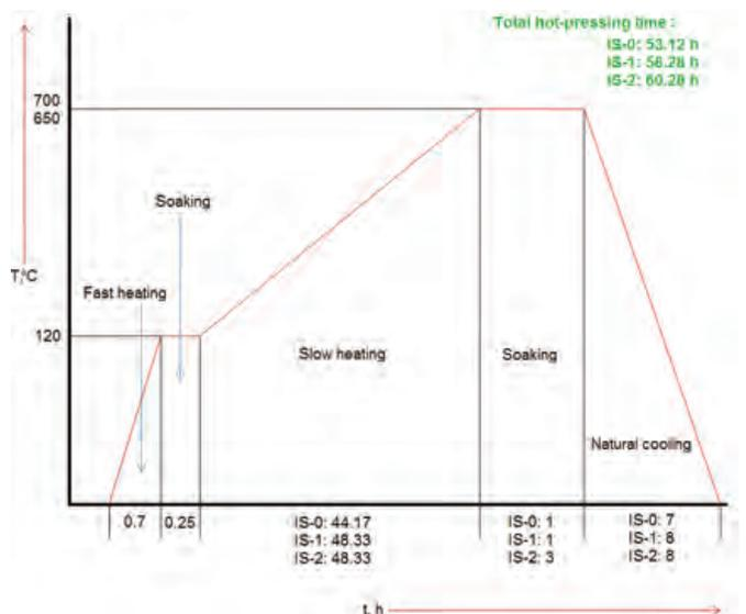
Figure 3. Hot-pressing plan for all the samples.
