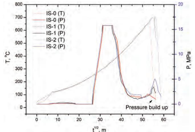
Figure 7. Pressure and temperature vs time profile of compacts.
