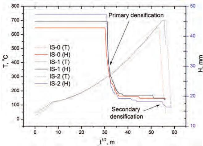
Figure 9. Height and temperature vs time profile of compacts.
