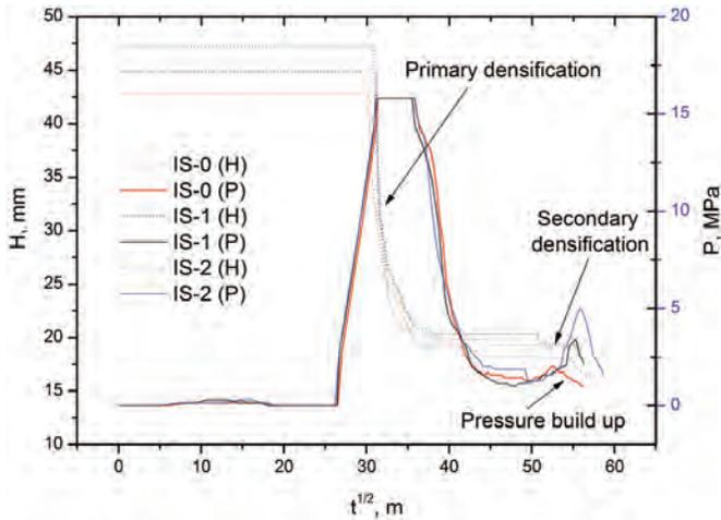
Figure 8. Height and pressure vs time profile of compacts.
