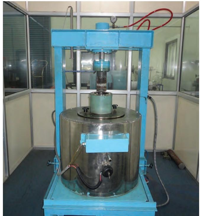
Figure 2. Custom built hot press used in the processing of composite samples.
