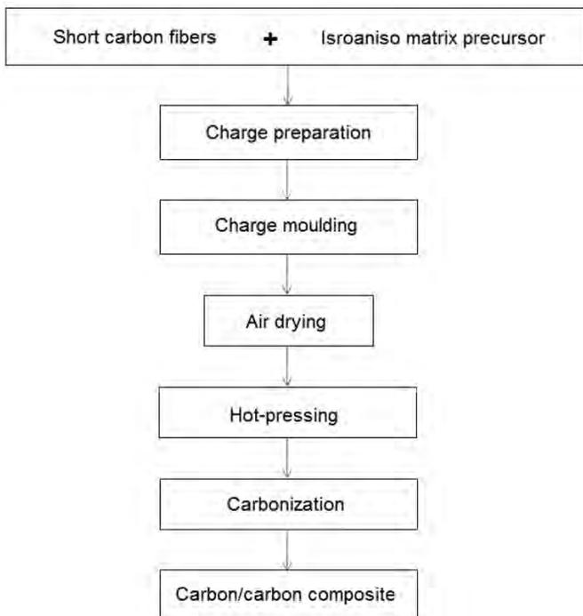
Figure 1. Schematic representation of process flow chart.
