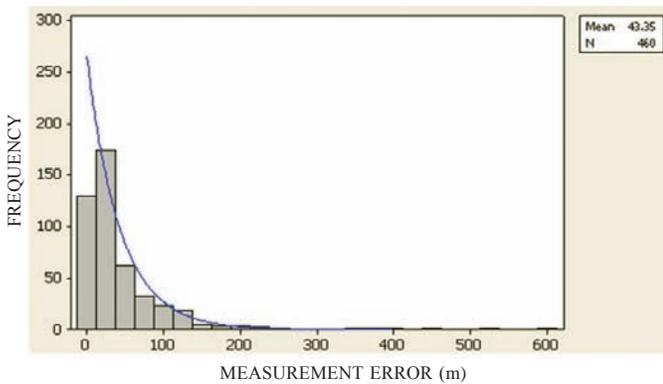
Figure 9. Histogram of POB measurement error (N=460 runs).
