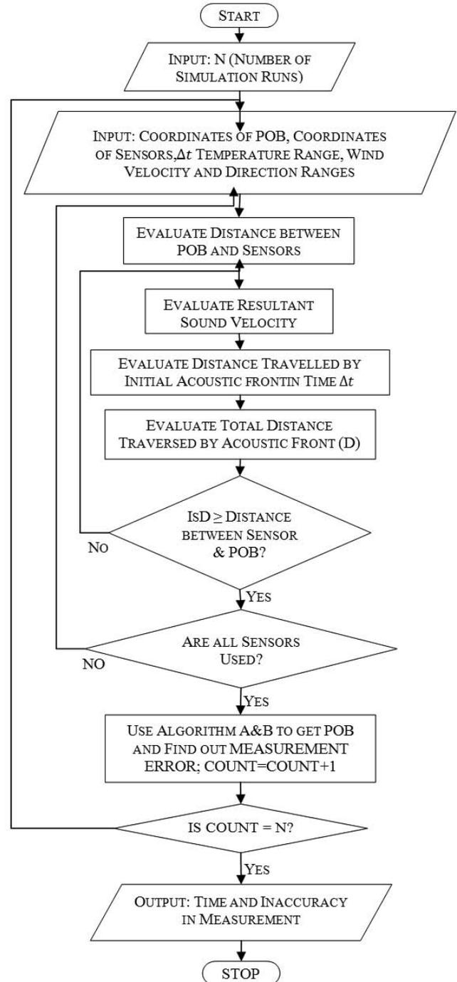
Figure 7. The flowchart of the simulation scheme.
