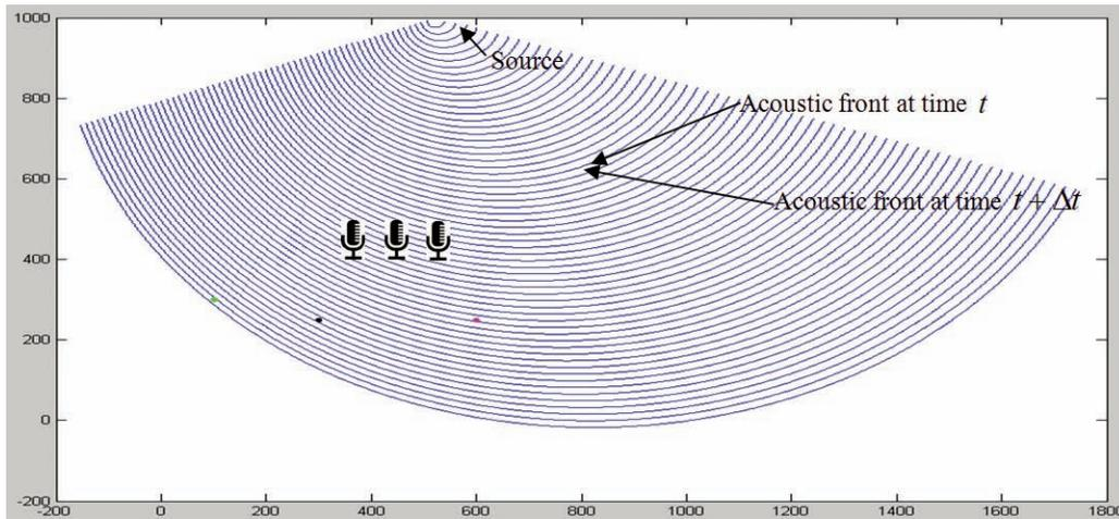
Figure 8. Simulated acoustic front of explosion approaching the sensors.
