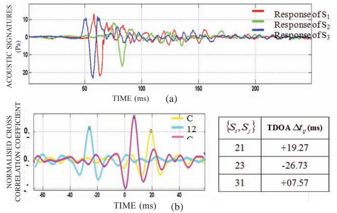
**Figure 11. (a) Acoustic signatures (b) cross correlation of three acoustic sensors.**
