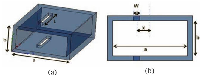
Figure 1. A slot doublet on the broad wall of a waveguide: (a) 3D view and (b) front view.
