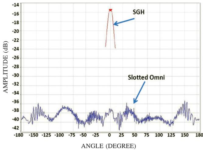
Figure 8. Gain measurement of antenna at 38 GHz.
