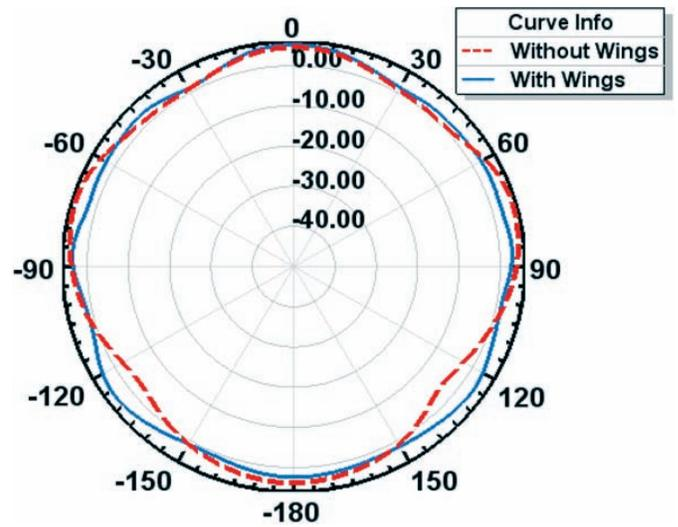
Figure 3. Comparison of Az pattern of antenna.
