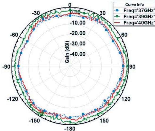
Figure 9. Measured Az pattern of antenna.
