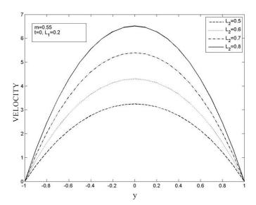
Figure 4. Steady state velocity for different values of  $L_2$  with time t=0.
