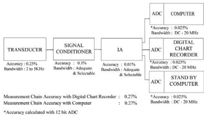
**Figure 3. Measurement chain and data acquisition in early 1990s.**
