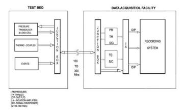
Figure 1. Components of instrumentation measurement system.
