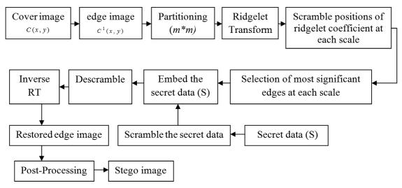
Figure 4. Block diagram of proposed steganography system.
