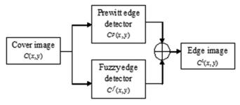
Figure 3. Block diagram of proposed hybrid edge detector.
